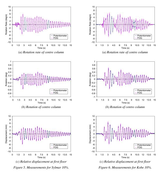
Whereas displacement measurement using the conventional transducers is readily available in a laboratory environment, it is almost impossible in an actual earthquake scenario. In contrast, for applications of the FOG, there is no difference between the displacement measurement in a laboratory experiment and that in a tall building structure.
